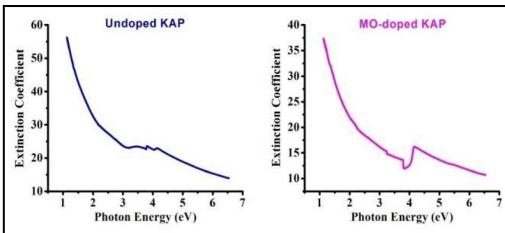
Figure No.4: (C) Plot of photon energy vs extinction coefficient for Undoped and Methyl Orange doped KAP crystal
