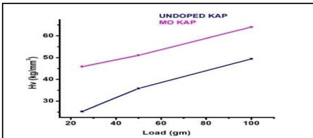
Figure No.6: Load vs  $H_v$  plot of Undoped and methyl orange doped KAP crystal
