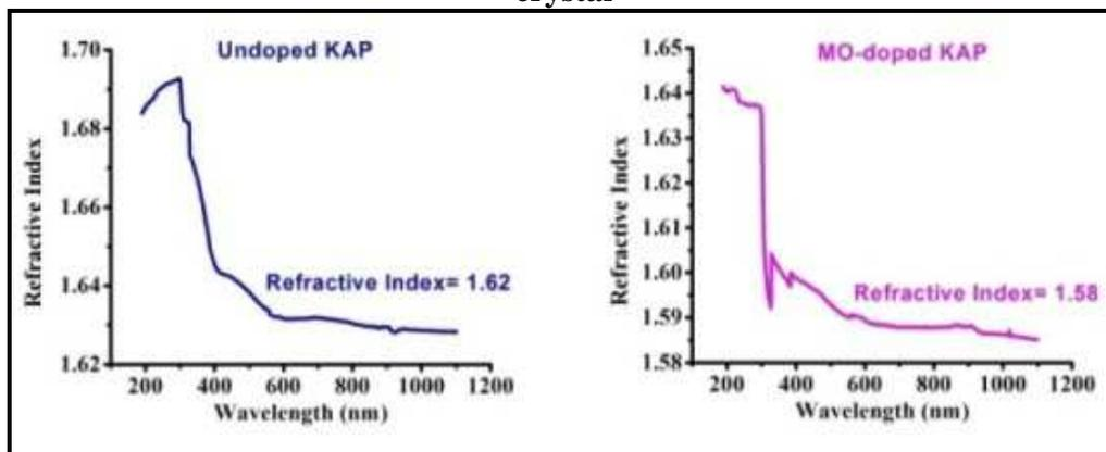
Figure No.4: (E) Plot of wavelength vs refractive index for Undoped and Methyl Orange doped KAP crystal
