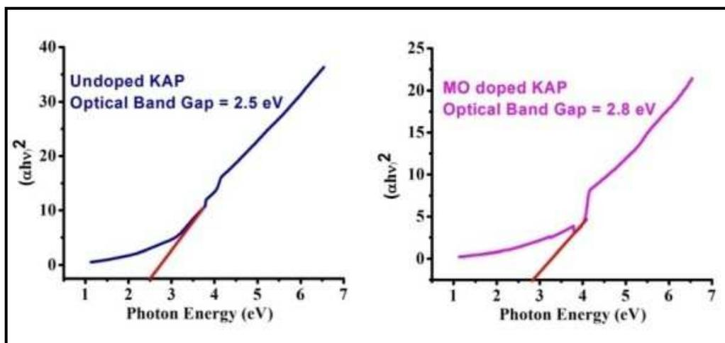
Figure No.4: (B) Tauc's plot for Undoped and Methyl Orange doped KAP crystal
