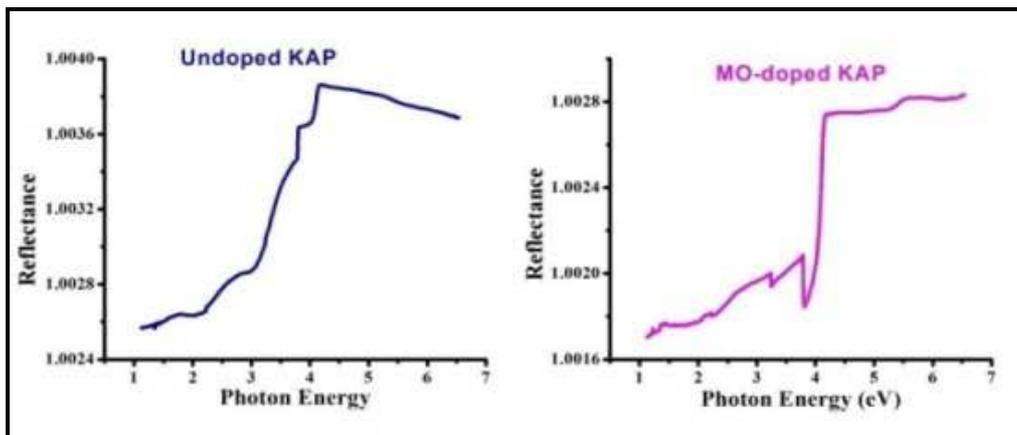
Figure No.4: (D) Plot of photon energy vs reflectance for Undoped and Methyl Orange doped KAP crystal
