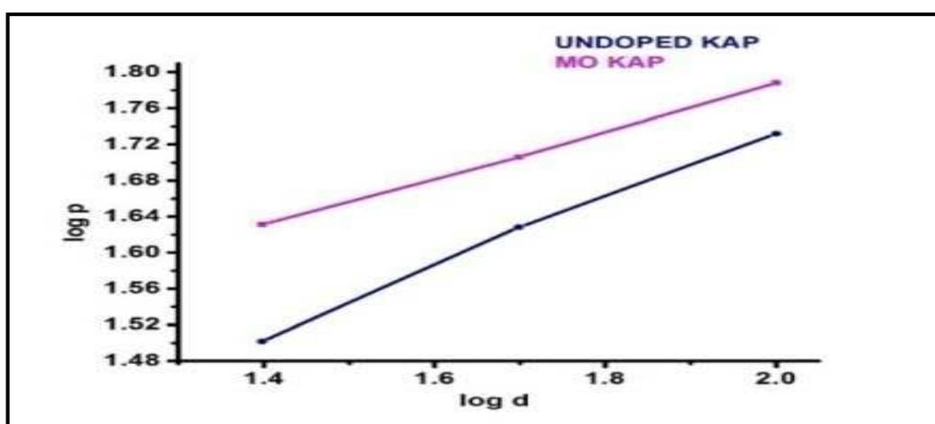
Figure No.7: Log  $p$  vs log  $d$  plot of Undoped and methyl orange doped KAP crystal
