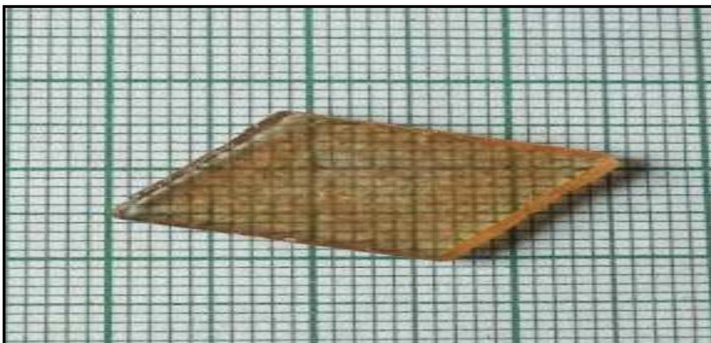
Figure No.1: As grown Methyl Orange doped KAP crystal
