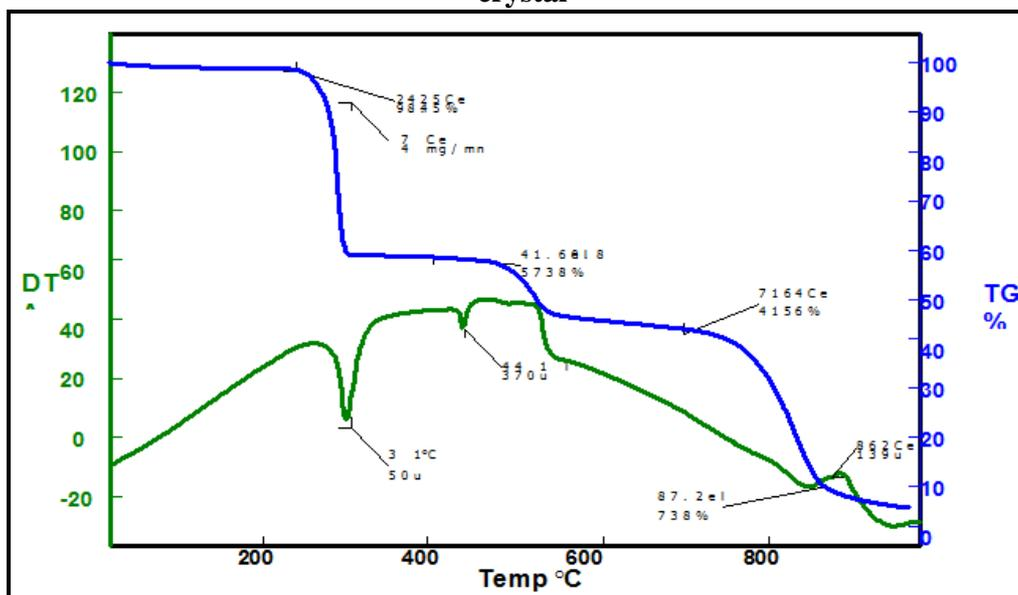
Figure No.5: TG/DTA thermo gram of methyl orange doped KAP crystal
