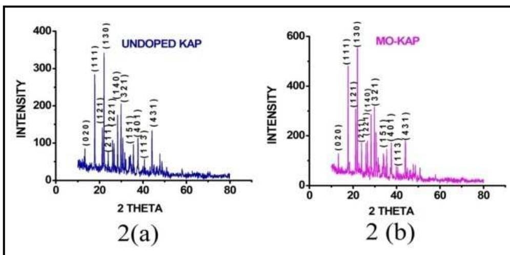
Figure No.2: Powder XRD pattern of (a) Undoped KAP (b) MO-KAP
