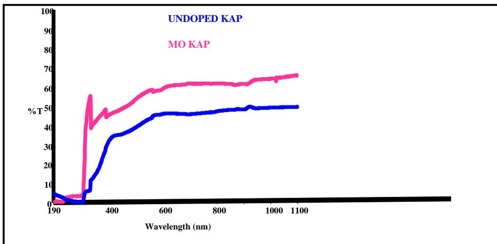
Figure No.4: (A) UV-Transmission spectrum of Undoped and methyl orange doped KAP crystal
